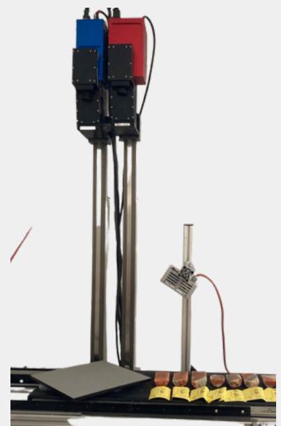
Figure 1: Scanning of the samples using the HySpex lab setup with both VNIR and SWIR cameras.
