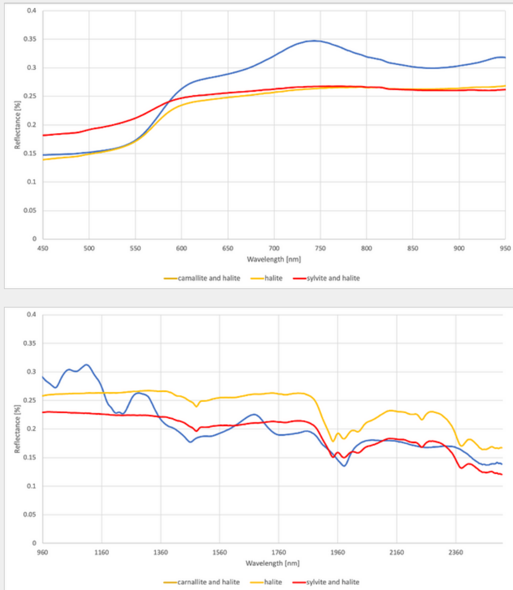
Figure 3: Top: VNIR, Bottom: SWIR spectral plot of the three main lithologies
