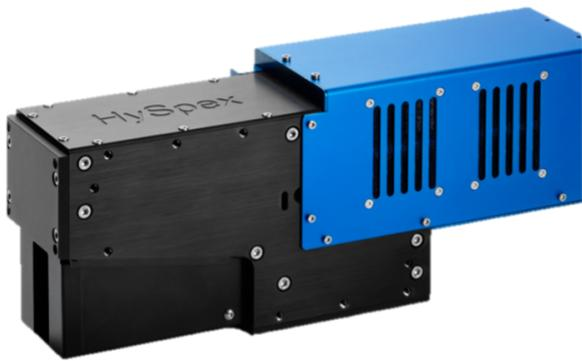
The thin film samples were scanned using the **HySpex VNIR-1800 hyperspectral camera** and a broadband halogen illumination source. The camera covers the spectral region of 400-1000nm with a spectral resolution of 3.26nm and a spatial resolution of  $60\mu\text{m}$ . Featuring low background noise, high dynamic range, and superior signal-to-noise ratio, this state-of-the-art camera guarantees high-quality image data and the reliability needed for thin film analysis.
