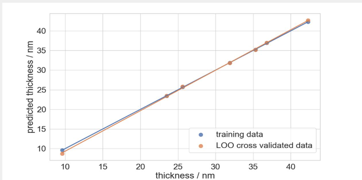
**Figure 3:** Thin film thickness values predicted by the PLS regression models trained using the complete dataset (blue) and using Leave-One-Out Cross Validation (orange) plotted against the measured reference value.
