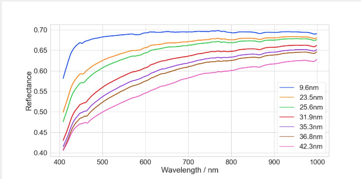
**Figure 2:** Mean reflectance spectra for all 7 samples (same color coding as in Figure 1). Changes in film thickness result in a change in spectral properties of the coating.
